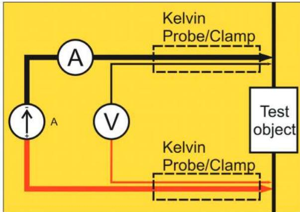
The Kelvin probes (incl. in BD-59090) are used for a 4 wire Kelvin test. This is a way of measuring continuity resistances ensuring all contact and lead resistances are compensated for which allows a much greater accuracy in measurements. Each Kelvin probe assembly has two probe tips. One tip is for the current generated and the other will measure the very small voltage present.
