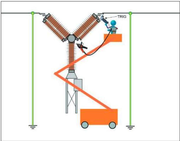
Measurement on CB with both sides grounded, DualGround. Here is a combination of one clamp and one probe used.
