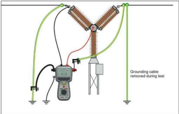
Traditional measurement from ground. Injection is done through existing grounding cable (earthing). Use any of the optional cable kits, GFL-00380/82/84, with 5, 10 or 15 m cables.
