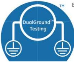
Equipment and methods that supports DualGround™ testing are associated with the DualGround symbol. This symbol certifies the use of groundbreaking technology and methods that enables a safe, fast and easy workflow with both sides grounded throughout the test.
