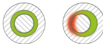
*The lubricating film in a bearing is very thin. A machine poorly aligned, or a foundation not supporting the machine in a proper way, will cause increased pressure and overheating of the lubricating film. This will in the end destroy the lubricant, and cause the machine to fail.*
