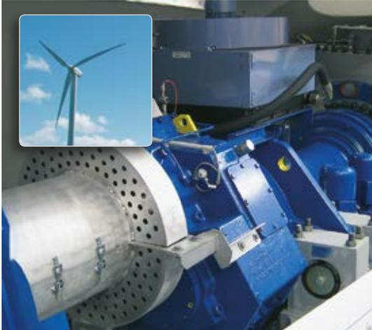
Easy-Laser® is used to align generators and gearboxes in wind turbines of a number of sizes and makes. Special brackets are available (accessories) for alignment with locked rotors, which increases the safety for the operator.
