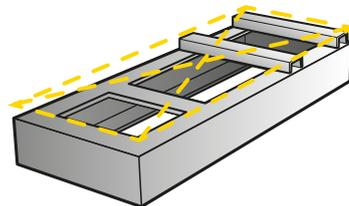
*A foundation has to be flat within 0.1 mm/1000 mm to be able to do its job as intended. 0.1 mm is the same as the thickness of a human hair!*
