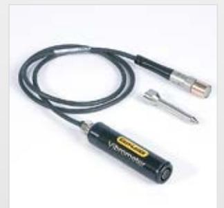
E285 Vibrometer probe. For measuring vibration and bearing condition. For connection to display unit, one of the red cables of system E720/E710 is used. Part No. 12-0656
